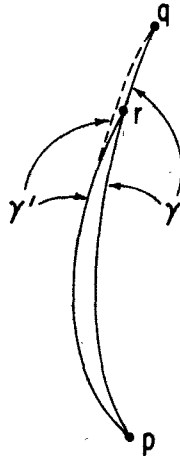
Fig. 9.3. A spacetime diagram illustrating the fact that if a timelike geodesic \gamma connecting points p and q has a point r conjugate to p lying between p and q , then a nearby timelike curve \gamma' connecting p and q can be constructed which has greater elapsed proper time than \gamma (see theorem 9.3.3).
